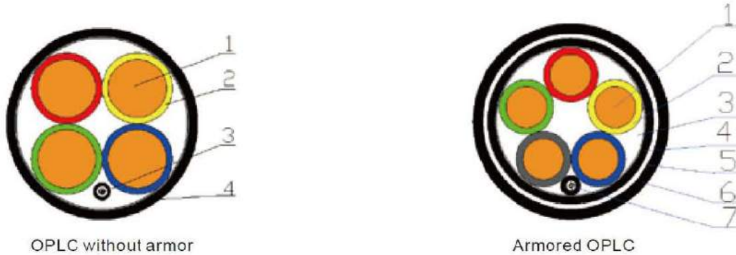
Figure 1 1—conductor 2—insulation 3—optical unit 4— sheath
